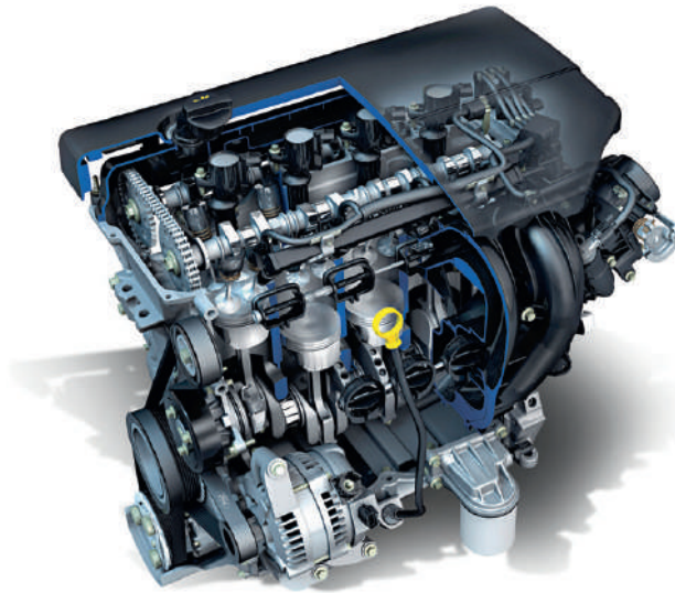
Figure 2.94 Valves in position on a cutaway engine. (Source: Ford Media)
